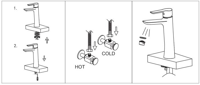
4. Re-install the rubber washer followed 5.Attach flexible hose to water supply. by the metal washer and lock-screw. Using the wrench to tighten lockscrews.
