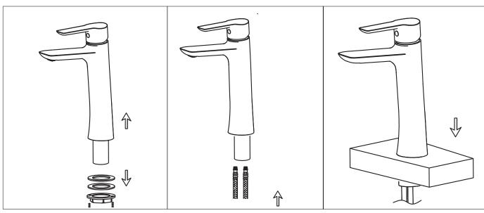
1. Remove the rubber washer, metal washer and locking screw from the faucet. cold flexible hoses to the faucet.DO
